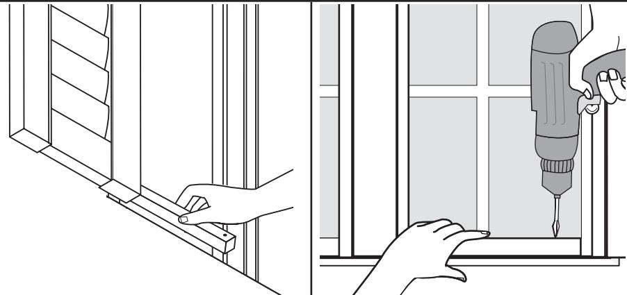
With shutters open, place light blocks in the light gaps, predrilled holes up. Secure the light blocks using 1-1/4" screws. You may wish to turn the light block upside down and secure with a nail gun.
