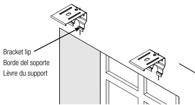
Place bottom groove of cassette into bracket lip and push. Snap into place.
