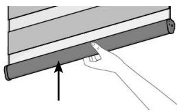
To lower: gently pull straight down using the hem bar grip. Lower shade to the desired position.
