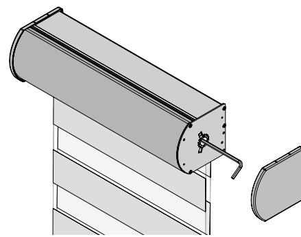
The shade brake is calibrated at the factory, but if the shade creeps down or is difficult to lower once installed, the brake may be adjusted. To do so, gently remove the end cap on the right side of the shade and insert a  $5/32"$  Allen wrench. If the shade creeps down, turn the wrench clockwise  $1/4$  turn to tighten the brake. If the shade is difficult to lower, turn the wrench counterclockwise  $1/4$  turn to loosen the brake.
