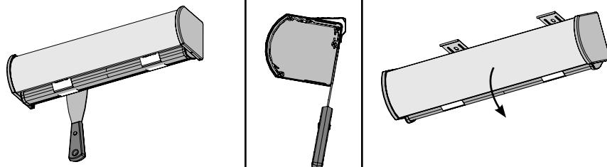
To remove shade from brackets, push in on bottom to release shade. This may require pressure. Rotate down.
