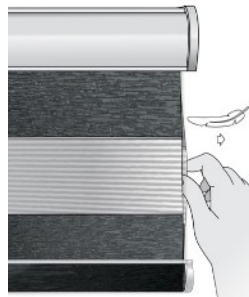
Figure 5: Correcting unaligned fabric
